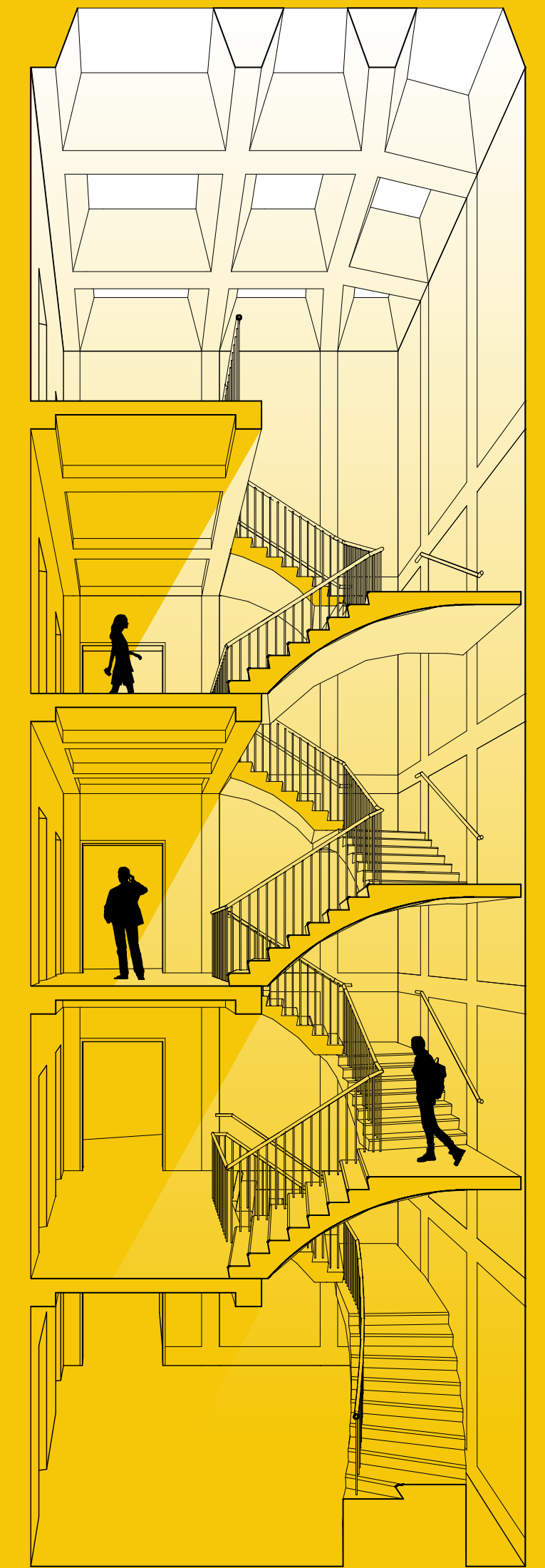
Roof lights and shallow treads make using the stairs effortless and enhance your journey through the building
